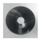
R1 – METRIC SLITTING SAWS FINE PITCH TO DIN 1837 TOOTH FORM A DIN1840 Dimensions in millimeters. Used for shallow cutting and cut-off operations. Hollow ground on both sides to prevent binding. To order please email or phone the details below, we accept card payment and provide next day delivery in the UK. For larger quantities we offer a discounted price. For special cutters please email or phone for a quote.
