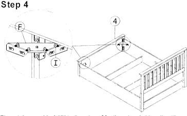
Fix metal corner block 'F' to the edge of footboard and side rails with bolts 'I' as shown
