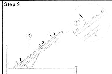
Assemble the bed base on the right & left hydraulic frame and fix bolts starting from '1' to '3' as shown.
