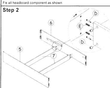
Assemble the left & right side rails to the center storage panel with minifix screws as shown.
