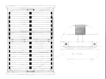
Adjust the bed base, make sure distance with the front footboard approximately 10 -15mm gap as shown.
