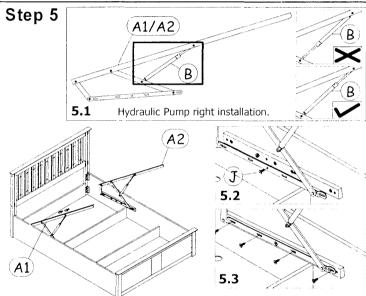
Firstly, fix the hydraulic pump to each hydraulic base as shown in diagram 5.1. Next, fix the left & right hydraulic support to the both side rails. Then, fix bolts 'J' first as shown in diagram 5.2 and do not tighten yet. Finally, fix all bolts and tighten as shown in diagram 5.3.
