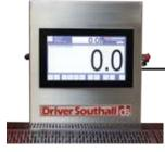
15.6" Full colour, easy clean, touch-screen display with multi-level password access, presenting an array of statistical and graphic data
