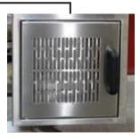
Reject bin door sensing with electronic access via HMI Reject confirmation and bin full sensors Fully compliant to supermarket COP's
