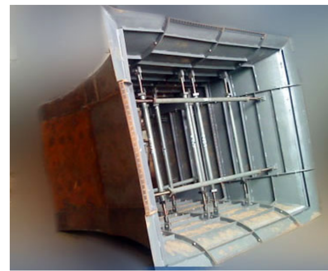
Bell Mouth Formwork
