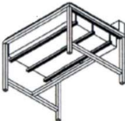
A uni-strut/all thread system works well for large sinks that will have a lot of weight in them. Please consider the application and support accordingly. Scientific Plastics is not responsible for damage caused by a sink not supported correctly.
