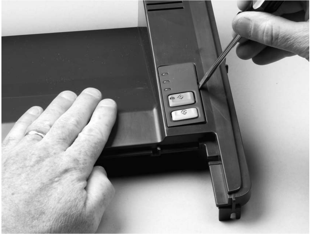
Figure 6-12. Removing the control panel (1 of 2)
