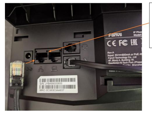
**3.9** – This is where one end of the Ethernet cable will be plugged into.
