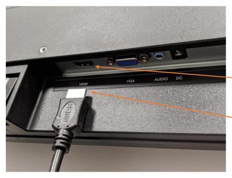
**2.11** – This is the HDMI input for the Monitor. This is where the HDMI cable will be plugged into.
