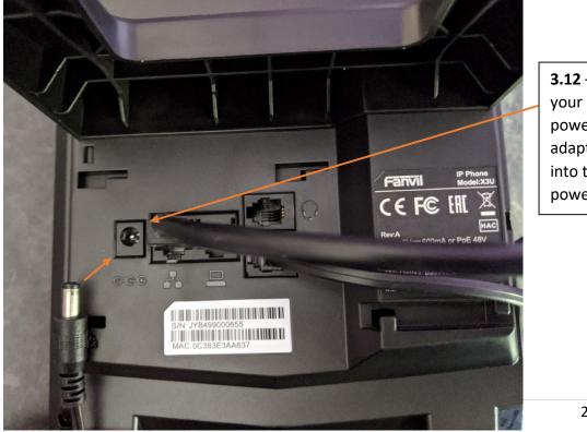
**3.12** – Plug your phone's power adapter cable into this power input.
