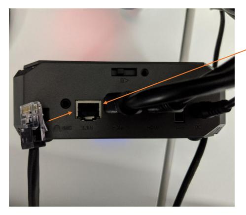
**3.10** – Plug your Ethernet cable into the "LAN" port on the PC.
