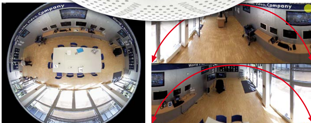
The ceiling-mounted c25 delivers two 180° panorama images of a room.
