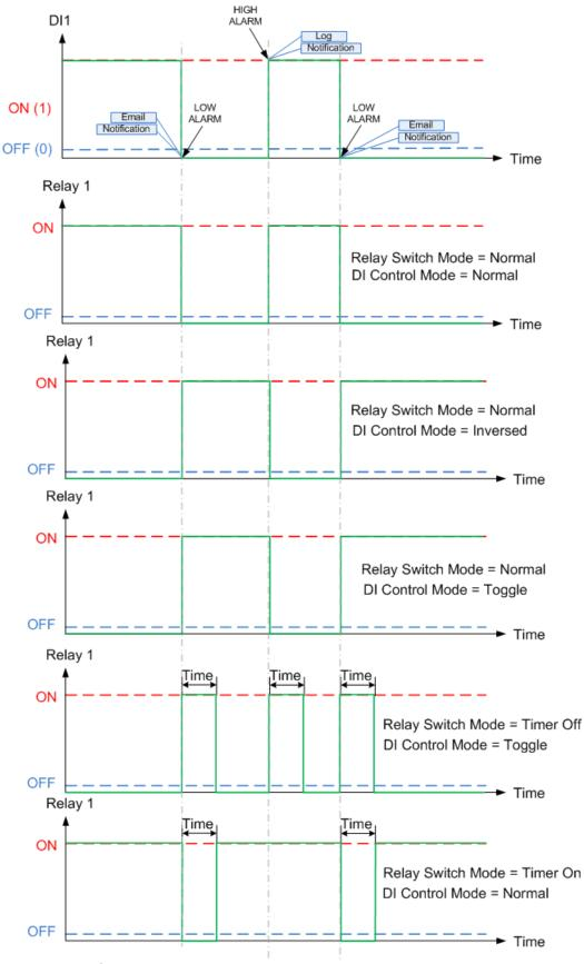
Figure 10.18. Digital input controlling relay examples
