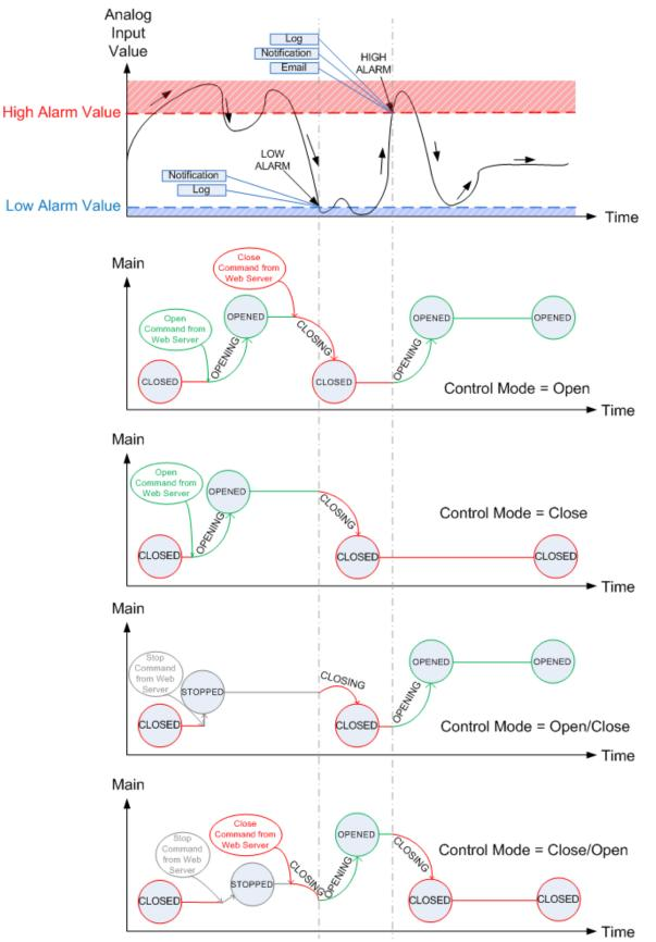
Figure 10.23. Analog Input controlling Main Controlled Device examples
