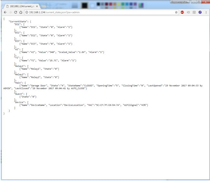
Figure 11.3. JSON response from smartDEN Opener
