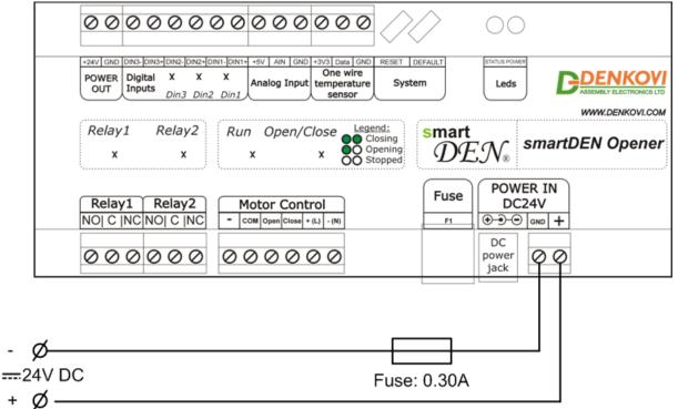
Figure 6.13. 24VDC Power Supply
