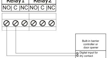
Figure 15.1. Hardware Connection to smartDEN Opener
