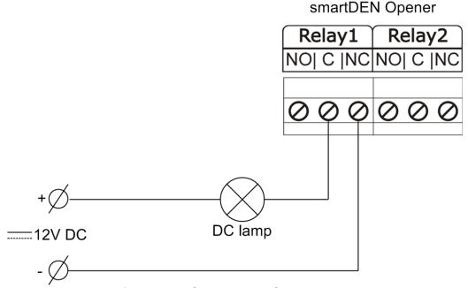
Figure 6.6. Controlling DC load with relay
