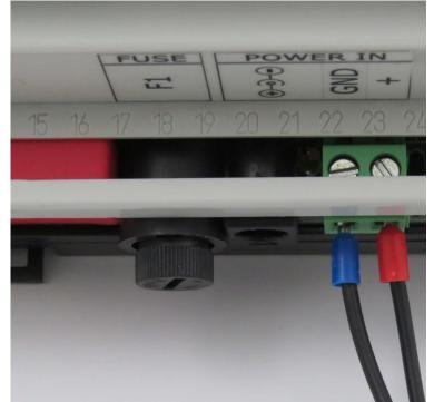
Figure 6.14. smartDEN Opener power supply using terminal wires
