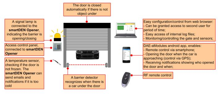
Figure 2.2. Controlling a garage door
