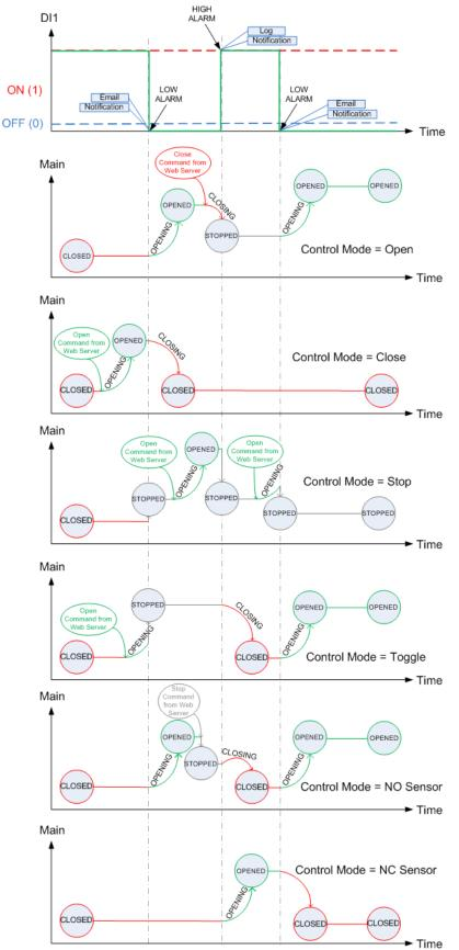
Figure 10.20. Digital Input controlling Main Controlled Device examples
