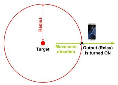
Figure 16.7. GPS Outside control by location
