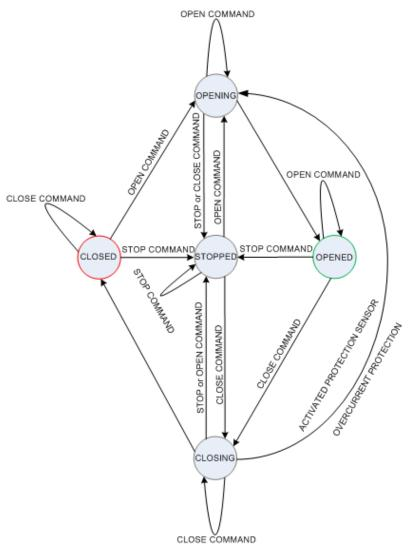
Figure 9.1. Graph of Main Controlled Device's states
