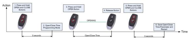
Figure 6.36. Open/Close Time programming via RF Remote Controller
