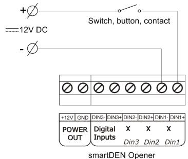
Figure 6.8. Connecting digital inputs using external power out
