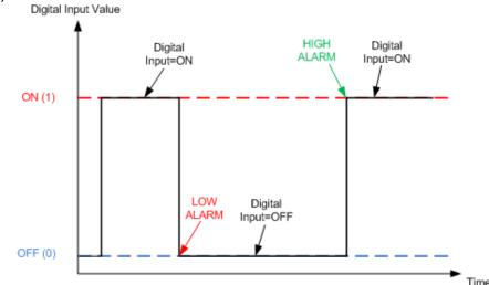
Figure 10.16. Digital Inputs alarms
