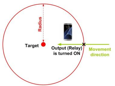
Figure 16.6. GPS Inside control by location
