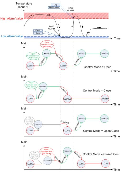
Figure 10.28. Temperature Input Controlling Main Examples
