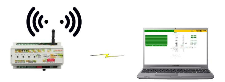
Figure 6.18. Connecting to smartDEN Opener's Wi-Fi network. This is the initial connection
