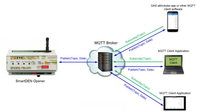
Figure 12.1. MQTT communication Overview
