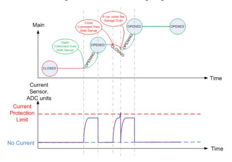
Figure 10.13. Current protection usage example
