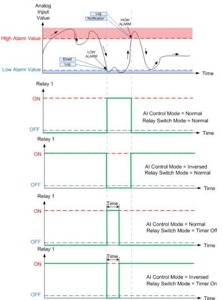
Figure 10.25. Analog Input controlling "Relay 1" examples
