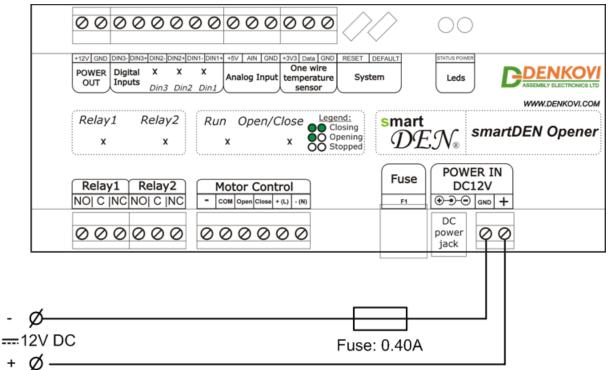
Figure 6.12. 12VDC Power Supply
