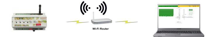
Figure 6.19. Connecting smartDEN Opener to a wireless router
