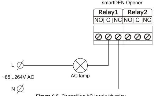
Figure 6.5. Controlling AC load with relay
