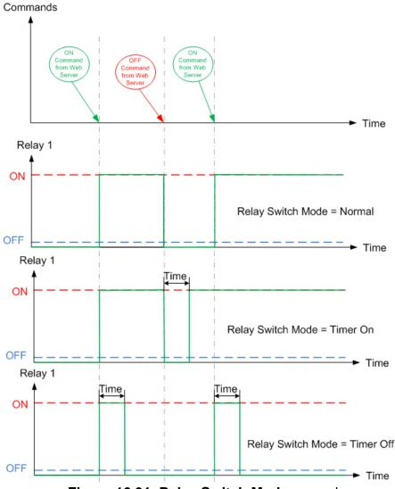
Figure 10.31. Relay Switch Mode examples
