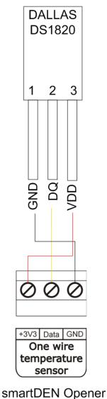
Figure 6.11. Connecting one wire temperature sensor
