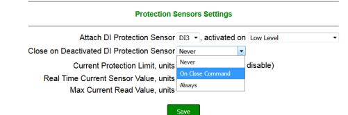
Figure 10.11. Close on Deactivated DI Protection Sensor options
