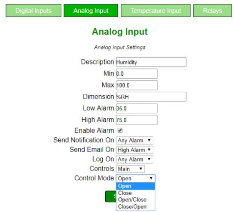
Figure 10.22. Analog Input controlling Main Controlled Device settings
