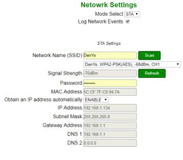
Figure 10.35. Station (STA) network mode
