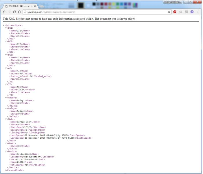
Figure 11.2. XML response from smartDEN Opener
