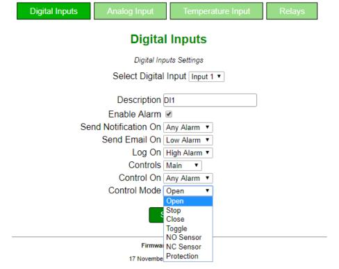
Copyright © 2017 Denkovi Assembly Electronics LTD Figure 10.19. Digital Input controlling Main Controlled Device settings
