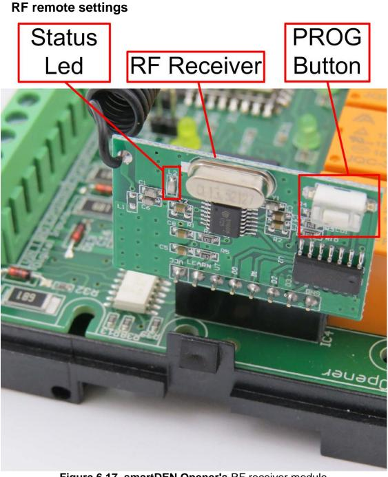
Figure 6.17. smartDEN Opener's RF receiver module
