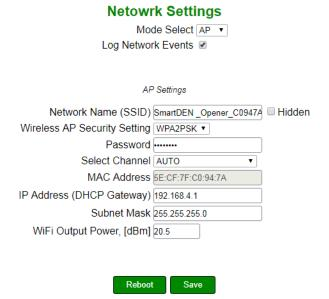
Figure 10.34. Access Point (AP) network mode
