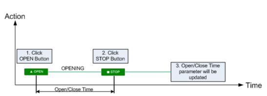
Figure 6.34. Setting Open/Close time via web server
