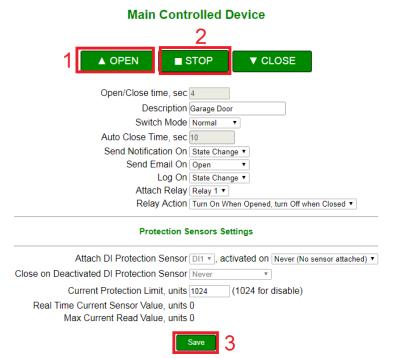
Figure 6.35. Setting the Open/Close time via web server
