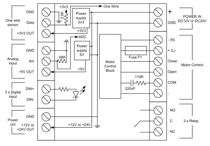
Figure 4.1. Internal block diagram of smartDEN Opener
