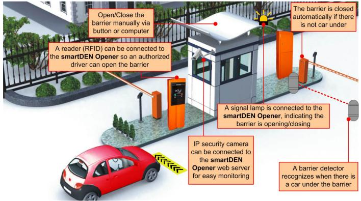
Figure 2.1. Controlling a barrier
