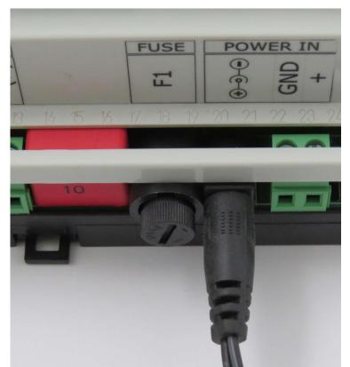
Figure 6.15. smartDEN Opener power supply using 2.5mm DC Jack
