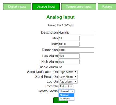
Figure 10.24. Analog Input controlling Relay 1
