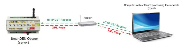
Figure 11.1. smartDEN Opener works as HTTP server
