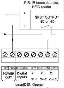
Figure 6.9. Connecting SPST output sensor
