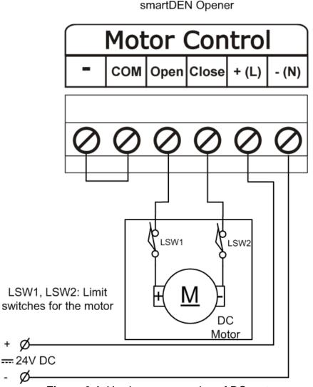
Figure 6.4. Hardware connection of DC motor
