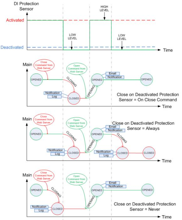
Figure 10.12. Close on Deactivated DI Protection Sensor options behavior
