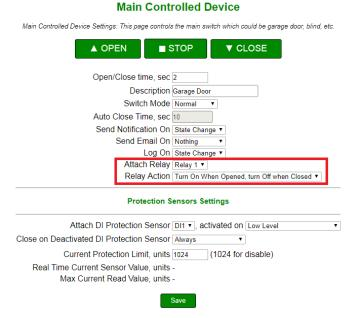
Figure 15.2. Configuration of Main Controlled Device
