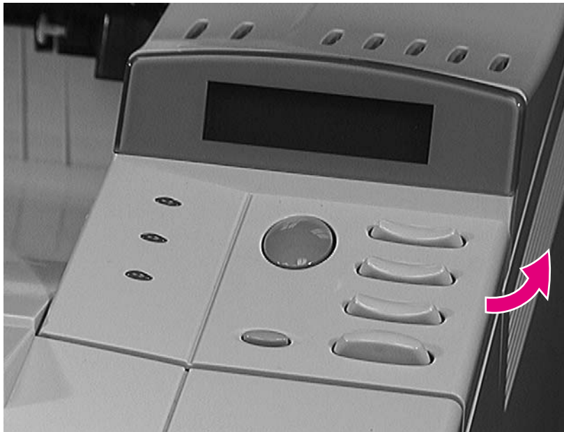
Figure 41. Removing the control panel overlay
