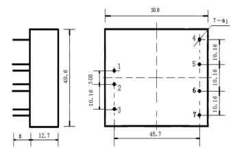
**Pin Definition** PIN Single Dual +Vin 1 +Vin 2 GND GND 3 REM REM 4 NC +Vo 5 0V+Vo 6 0V-Vo 7 TRIM TRIM
