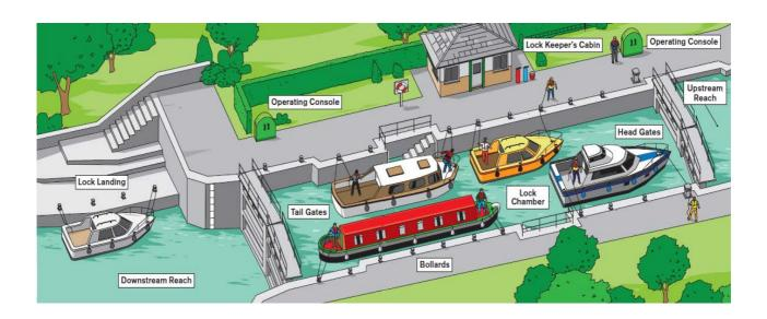
Not all of the locks on the river are the same. Some have wooden beams that have to be pushed open by hand. The others like this picture, are opened mechanically
