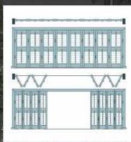
Rather than fitting shutters in the usual manner with frames and hinges, these shutters slide on a track.
