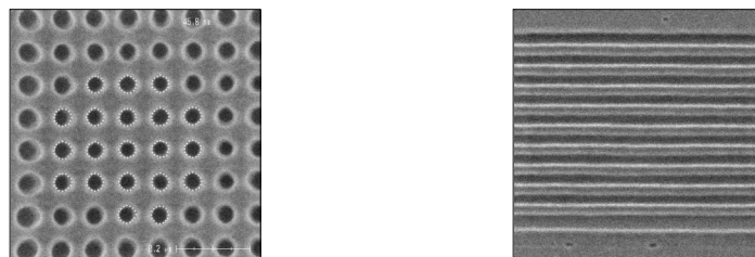
Figure 3. 45-nm CH/90-nm pitch (left) and 40-nm trenches/90-nm pitch (right) patterned on organic BARC using NTD.
