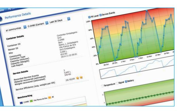
The fill level management and route planning SOTKIS is a system that uses an ultrasonic sensor and a web portal to provide information on the state of filling in each container.
