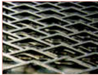
Expanded metal surface for excellent grip and drainage.
