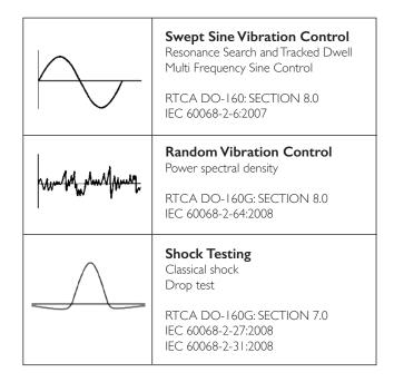
We can monitor product responses on up to 16 accelerometer channels as well as providing averaging algorithms for robust input control.
