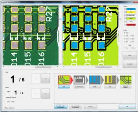
Using either Stencil Gerber, paste layer gerber or golden board programing is typically less than 5 minutes. Utilising our own proprietary gerber conversion software, Either online or offline. Full program transportability between
