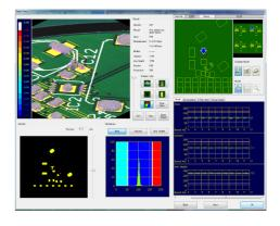
Using live SPC feedback, Process control and Studies can be easily implemented. SQL data storage either locally or on a remote server, And data export to Excel or CSV formats. Transition charts and histogram displays enable simple tuning of the print process. And to understand process indicators.
