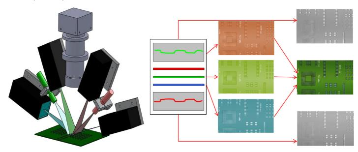
Our 5D post-print solder paste inspection process incorporates patented new sensor technology and simultaneously combines 3D and 2D image processing methodologies that deliver defect detection beyond that was previously possible.
