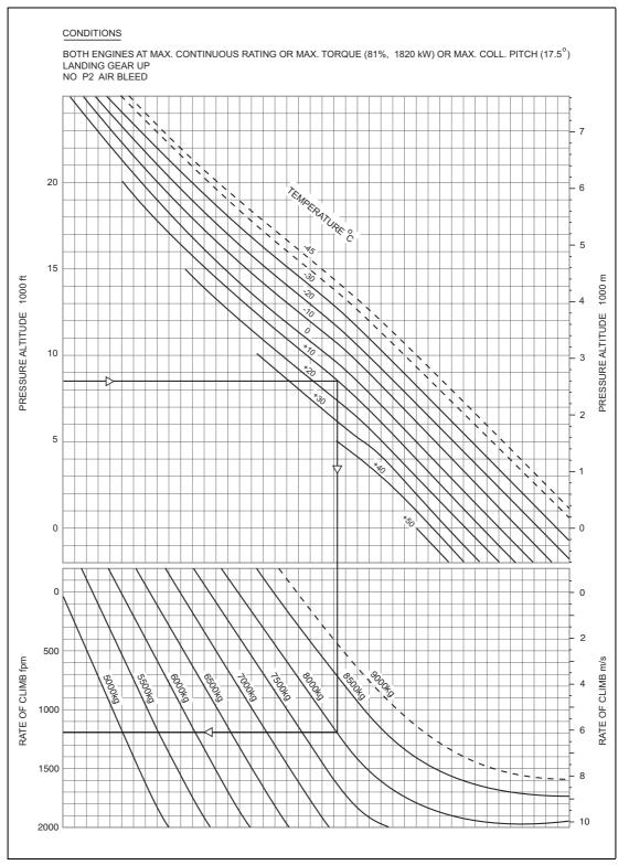
Figure 3.11 Rate of Climb at  $V_Y$  – Two Engines
