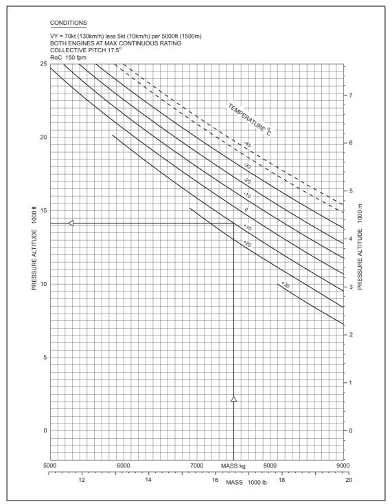
Figure 3.16 Service Ceiling – Two Engines
