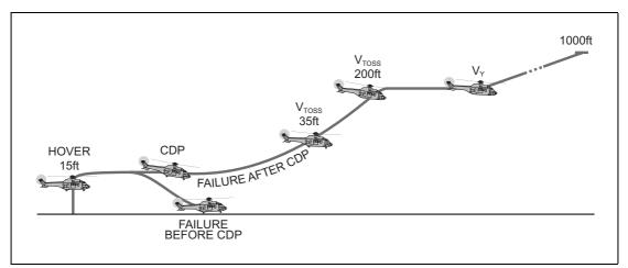
Figure 3.32 Engine Failure at Take-Off – Procedure No. 1
