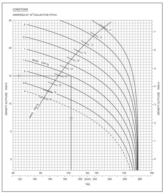
Figure 3.13 Airspeed in Level Flight – Two Engines
