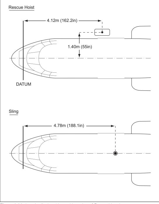
Figure 3.26 Longitudinal and Lateral Location of External Loads
