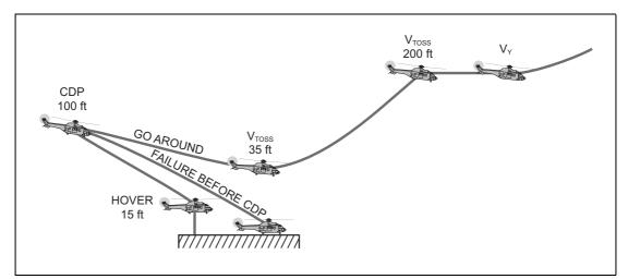
Figure 3.38 Engine Failure at Take-Off from Helipad
