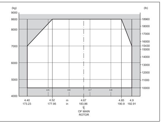
Figure 3.3 Longitudinal CG Limits
