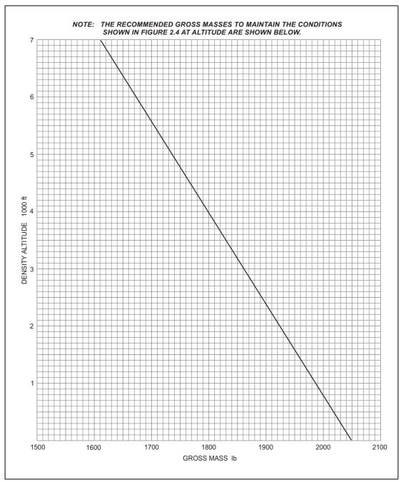
Figure 2.5 Gross Mass v. Density Altitude at Take-Off
