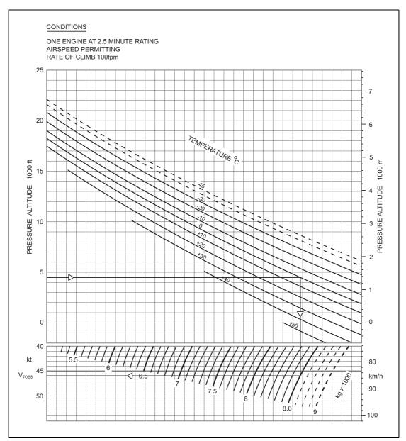
Figure 3.39 Take-Off Safety Speed (V<sub>TOSS</sub>) Determination
