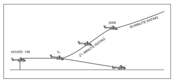
Figure 3.33 Engine Failure at Take-Off – Procedure No. 2
