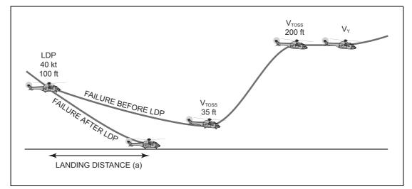
Figure 3.35 Engine Failure during Final Approach
