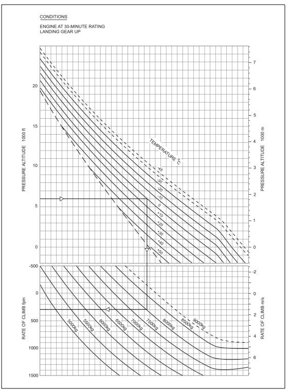
Figure 3.12 Rate of Climb at  $V_Y$  – Single Engine
