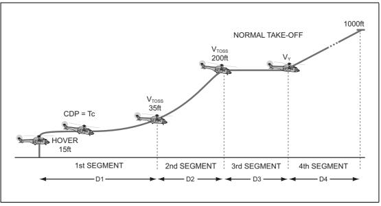
Figure 3.30 Normal Take-Off – Procedure No. 1
