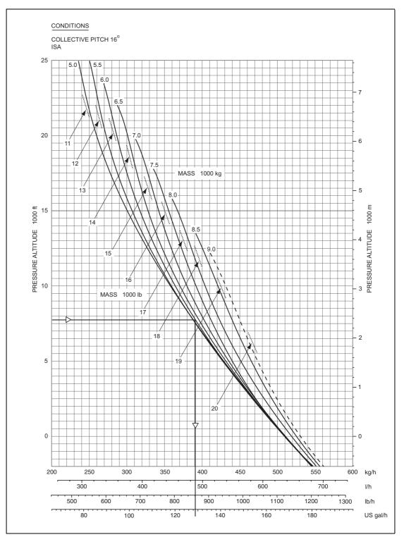
Figure 3.14 Hourly Fuel Consumption – Two Engines Cruise
