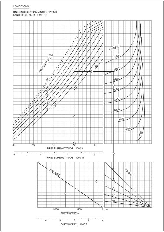
Figure 3.43 Determination of Distance D3 Required to Accelerate from  $V_{\text{TOSS}}$  to  $V_{\text{Y}}$  in Level Flight
