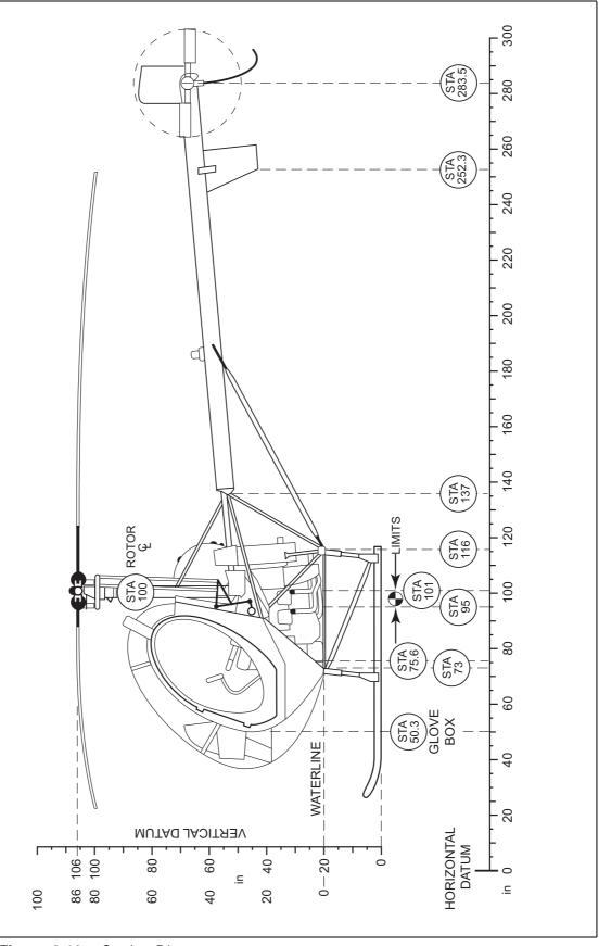
Figure 2.10 Station Diagram
