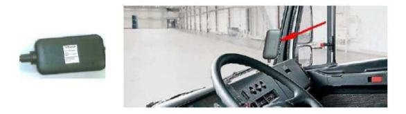
Please Note: The Geoloc is equipped with a 120 Ohm Can Resistor. The CAN wiring to CAN1 or CAN2 must take this into account!
