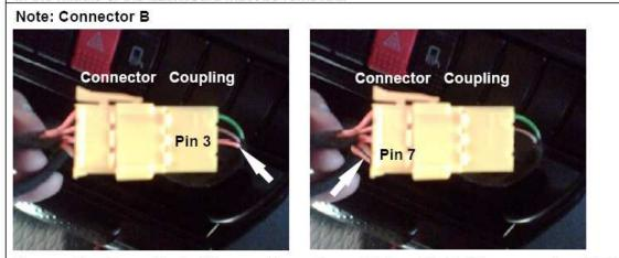
Remove the wire on Pin 3 of the coupling and mount this on Pin 7 of the connector which is free.
