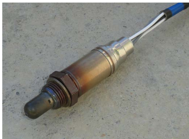
Figure 2.6 Lambda sensor for measuring flue gas O_2 content
