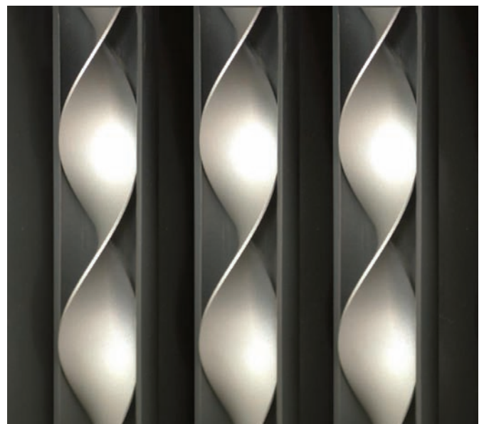
Figure 4.38 Cut-away showing turbulators in vertical firetubes
