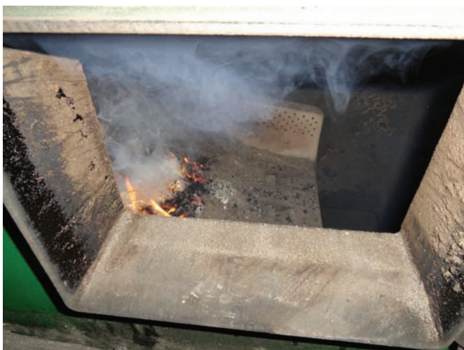
Figure 4.16 Unburned gases produced in slumber mode
