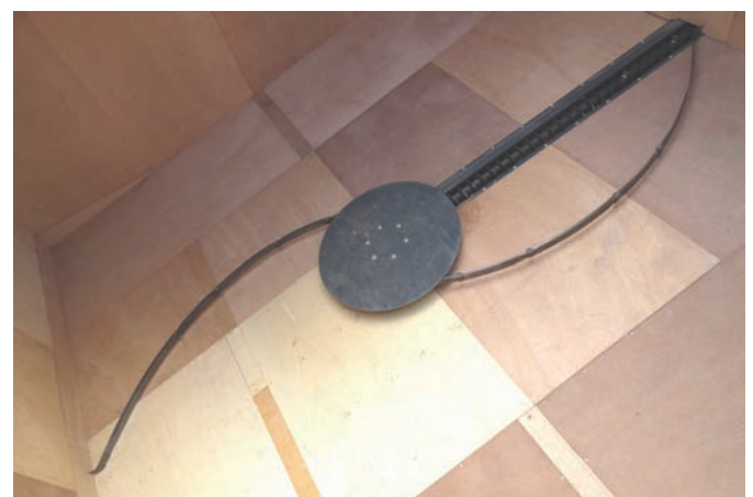
Figure 3.9 Sweeping arm extractor and fuel extract auger in a square silo
