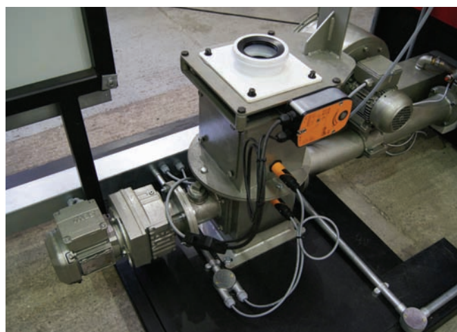
Figure 4.10 Underfed stoker auger mechanism
