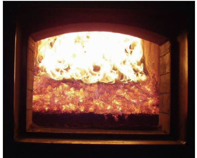
Figure 4.6 Combustion on a stepped grate
