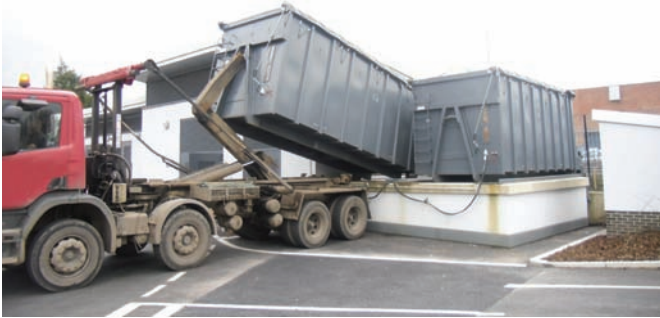
Figure 3.6 Hook lift container being delivered
