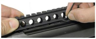
Once the rail is in place, secure it to the adapter with the two socket head caps screws and to the nuts in the front spacer with the three (#8-32) screws.
