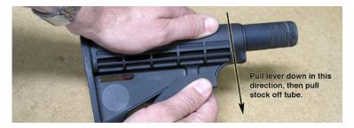
To install the M4 Carbine buttstock included in Mesa Tactical stock kits, ensure the stock lock nut and end plate end are installed on the stock receiver extension tube (see illustration).
