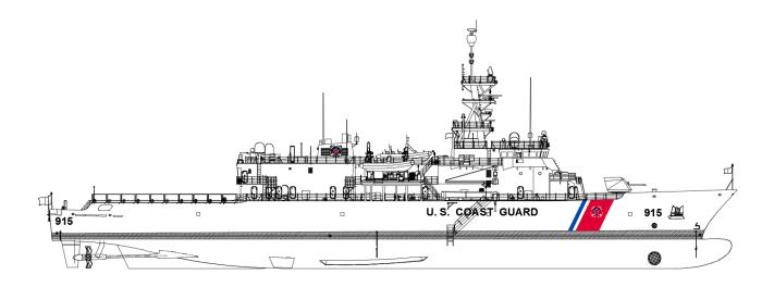
OPC Characteristics: •Length: 360 feet •Beam: 54 feet •Draft: 17 feet •Sustained Speed: 22 Plus knots •Range: 8500 Plus nautical miles •Endurance: 60 Days
