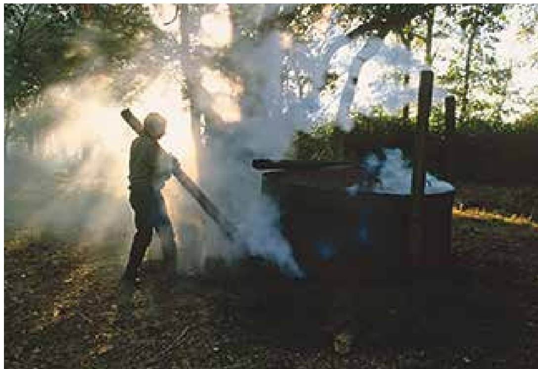
One hour into the burn process, Jim locates the chimneys and seals the lid.
