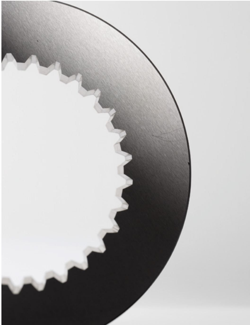
>> Cutting of a pattern for high precision gears (max. error: DIN 3962 Grade 3). First hole made with a DR2 drilling machine.
