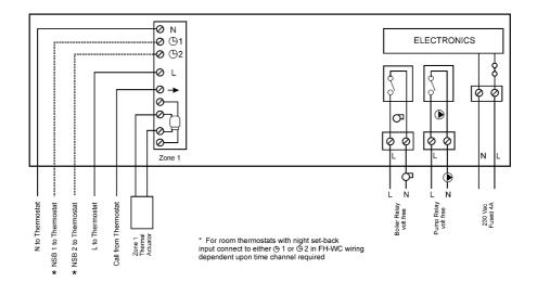
System 2: system with programmable room thermostats
