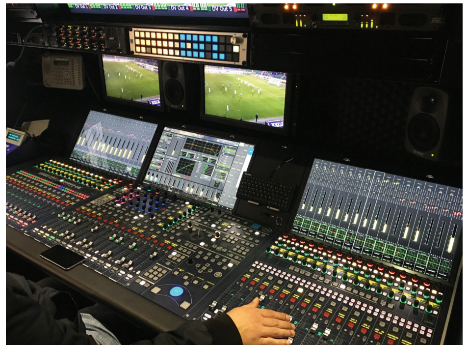
Italian production company NVP has equipped its OB 4 with solutions from Lawo, including mc 2 56 production consoles, a Nova router, and DALLIS interfaces, alongside the VSM control system and the V_pro8 video processing units.
