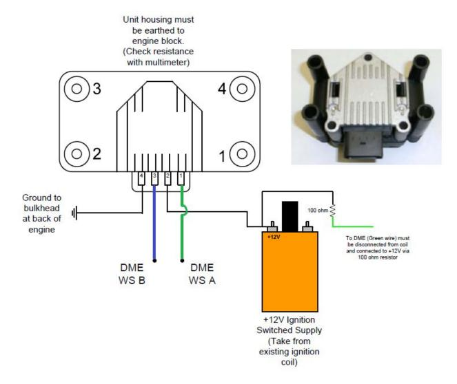
Note: Only early dash 944 models required the 100 ohm resistor as oval dash cars have a separate RPM output from the ECU to the dashboard.
