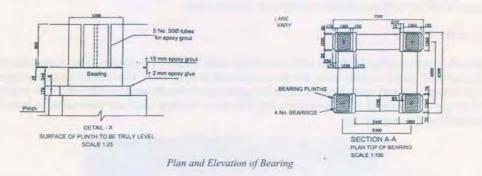
on top of each completed pier four elastomeric bearings were placed and a precast bottom slab for the pier (hammer) head unit, weighing 210t, was accurately positioned on the bearings. The web walls and the deck were the cast in place to complete the pier head unit, and this was temporarily tensioned down onto the four bearings by high strength bars anchored in the pier walls.
