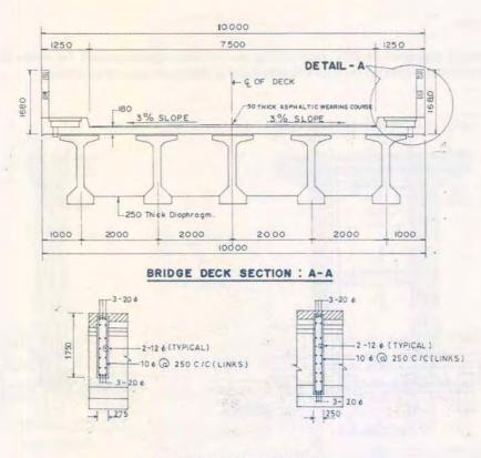
Schematic Details of Bridge Deck Section
