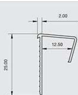
Locally manufactured from recycled plastic, Renderplas PVCu clip on edge beads / board stops are designed for plasterboard and cement board to provide protection to edges and a superior finish. On plasterboard at edges formed at door frames, windows and skirting boards or at a change of finish; on cement board at the exposed edge of the system
