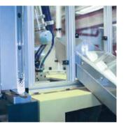
The robot is securely fitted to the injection moulding machine and can move over the mould and pull up the plastic items. This is done using a specially designed vacuum system which ensures that the sensitive items are not damaged.
