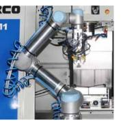
The robot opens both doors, puts in the raw material, tightens the machine's vice, removes it again after milling and puts it to one side.
