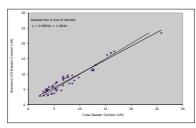
The IgA values ranged from 34.7 -621.1  $\mu$ g/ml on the Cube reader and 20.0-518.8  $\mu$ g/ml on the standard LFD Reader. The agreement between both readers was good, with the Pearson correlation r = 0.98 (95% CI, 0.96 -0.999) and with typical error of estimate 29.91 (95% CI 24.94 - 37.36)  $\mu$ g/ml, with slightly higher values on the Cube (mean 215.6  $\pm$  163.8) than the LFD Reader (148.3  $\pm$  142.1).
