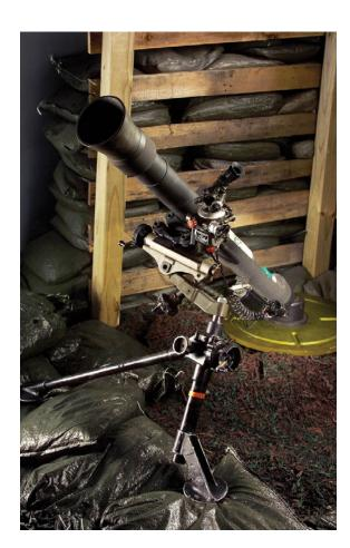
The mortar simulators provide sufficient recoil to disturb the operator's sight picture, requiring the trainee to achieve a proper aligned or compensated sight picture during each adjustment. In addition, the mortar realistically simulates weapon ballistics for each mortar simulator and round type, with scaled aiming posts provided.
