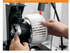
Most common reasons for interior blower failure are failures in the vehicle's electrical system, reduced flow in the air intake system and improper product handling during installation.
