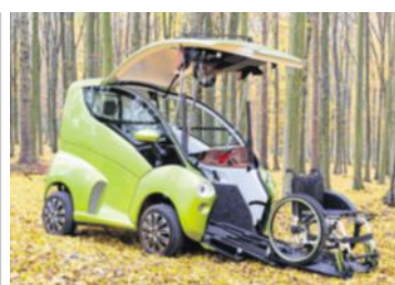
■ The Elbee: a front-loading car designed for disabled people
