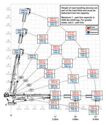
Weight of load handling devices are part of the load lifted and must be deducted from the capacity. Maximum 1-part line capacity is 4500 lbs. (2040 kg). For greater loads, use 2-part line.
