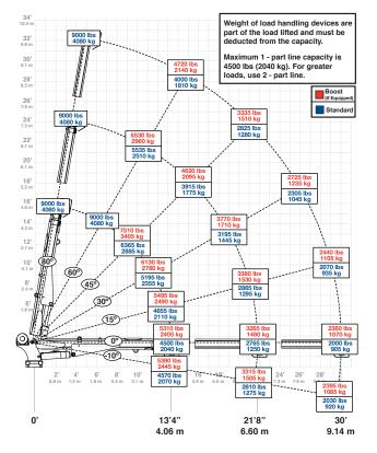
Weight of load handling devices are part of the load lifted and must be deducted from the capacity. Maximum 1-part line capacity is 4500 lbs. (2040 kg). For greater loads, use 2-part line.
