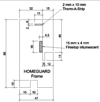
Seals may be interrupted at hinge and latch positions. Seals may be fitted in the door edge or reveal.
