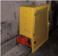
Guard installed over exposed bearing
