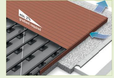
Closed gap with groove strip/P5 gap profile - raised construction ensures the required ventilation
