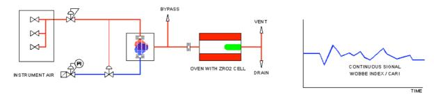
To convert the residual Oxygen percentage to a Wobbe Index value the analyzer is calibrated with two gases with known Wobbe Index values: a low calibration gas with a low Wobbe Index and a high calibration gas with a high Wobbe Index. Prior to calibration, the known Wobbe and CARI values are entered into the instruments software. When starting a calibration, the analyzer subsequently switches from sample to low cal. gas, high cal. gas and back to sample.
