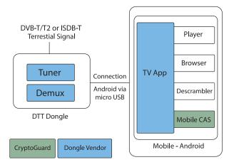
The figure shown is a high level configuration on how CryptoGuard Mobile CAS is implemented. CryptoGuard provides a Mobile CAS module which can run on an Android device.
