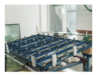
Acetal resin has high strength and hardness for a plastic material but is still much softer than steel so the bearings are only suitable for low loads and low speeds. In addition, they are not made to the same close tolerances as steel bearings so are classed as semi-precision. Acetal resin, PEEK, PTFE and many other plastics have low friction coefficients so our plastic bearings do not need to be lubricated.
