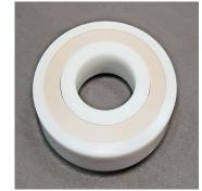
temperatures. SMB ceramic bearings are usually dry but we can lubricate them to order if required. Ceramic bearings with cages are stocked as open or with PEEK seals (2PKS). We can supply them with PTFE seals for extreme low temperature applications. Full complement bearings are only available open.
