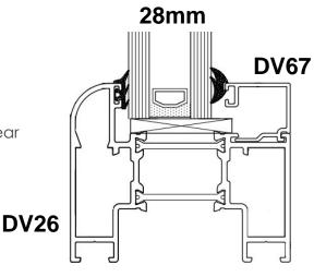
Bifolds incorporating the above specification of double glazing have an overall frame u'value of 1.8W/m<sup>2</sup>K, with a centre pane u'value of 1.2 W/m<sup>2</sup>K.
