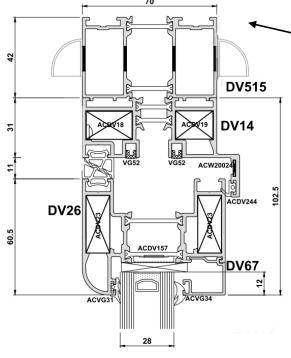
With the hood of the head vent fitted there is approx.12mm to the outer edge of the 42mm knock on
