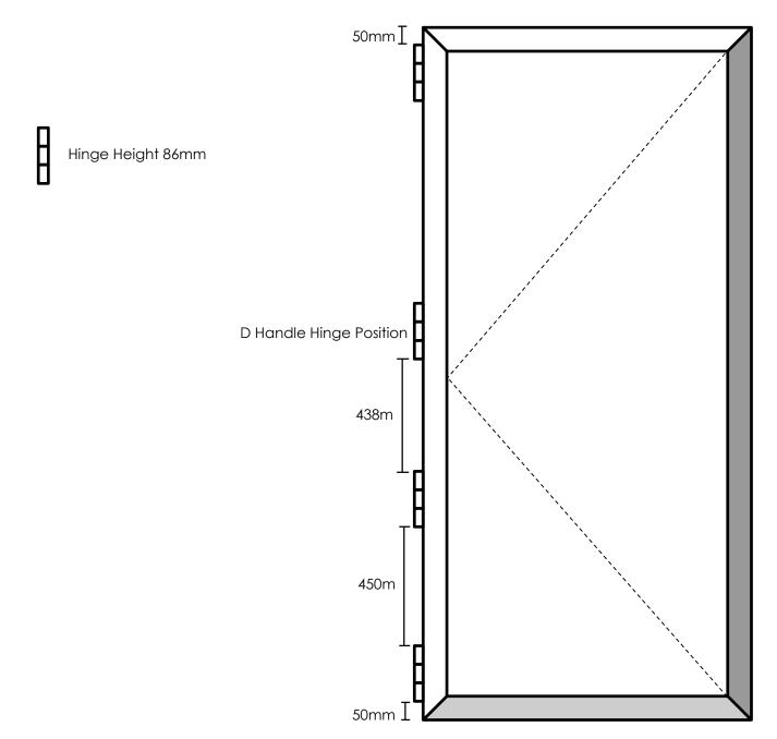
Each measurement is from the bottom/top of the profile to the bottom/top if the hinge as indicated
