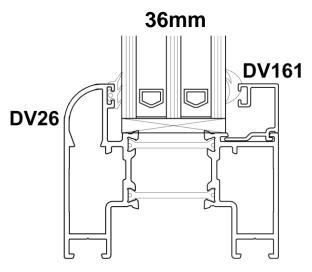
Bifolds incorporating the above specification of triple glazing have an overall frame u'value of 1.4W/m<sup>2</sup>K, with a centre pane u'value of 0.8 W/m<sup>2</sup>K.
