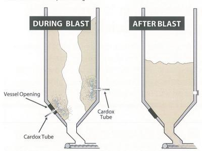
When recurrent build-up occurs in given location inside vessel (cone, discharge port, etc.) permanent fittings can be installed on the outside of vessel to accommodate Cardox Tubes.
