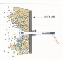
After achieving secure coupling, Tube is fired from a distance and build-up removed. Tube is then taken out and sealing plug put back nto place until another build-up occurs.
