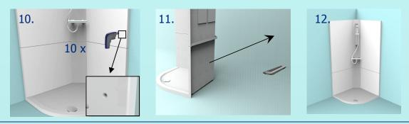
Install the waste fitting and screw the Envirotec Bathing Shower Enclosure to the walls taking care not to over tighten the screws (12). The shower door may now be installed according to manufacturers instructions (13) and can be attached directly to the Envirotec Leak free shower enclosure.
