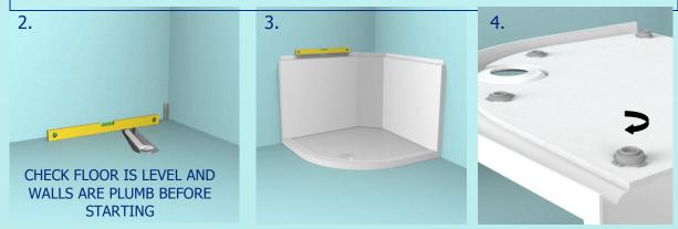
Place the tray section of the Envirotec Bathing Shower Enclosure into position and check for level along both walls (3). Also check that all feet are in contact with the ground (the tray should feel solid with no "spring" when tested). If adjustment is required, carefully turn the tray over using a soft blanket on the floor as protection and adjust the feet until correct floor contact is achieved (4).
