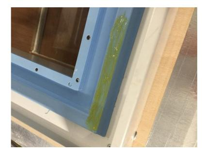
Figure 3 – Multi purpose grease provided for the IP6X test (NOTE: Image only shows part of the gasket, the full gasket was lubricated prior to testing).
