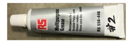
Figure 2 – Customer provided 'multi purpose' grease for the IP6X test only
