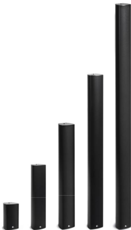
Specially developed for use in voice alarm systems, these loudspeakers are certified in accordance with EN 54-24 Type B. Weather resistant, passive, 100 Volt. Extremely even, targeted sound dispersion due to a complex multi-band crossover, a phase plug system and a passive Side-Lobe-Free functionality. Excellent levels of speech intelligibility, even in acoustically challenging venues with long reverberation times. Indoor and outdoor use.
