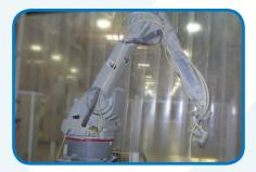
Each mold is recognized digitally to assure for proper tool temperature via heated water lines, for specific formulation blends and robotic pour patterns, creating the optimum setting for part reproducibility.
