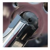
**Pic. 2:** Cutting tools finished with **MMP** TECHNOLOGY®, have significantly better surfaces than conventionally polished.
