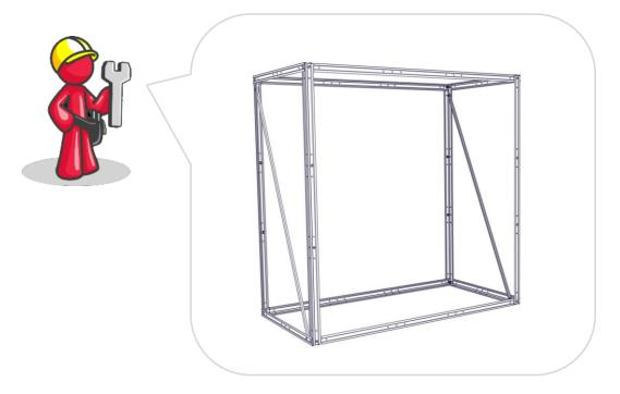
Step 3 – Bolt together the two end assemblies using horizontal sections
